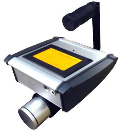
The NucScout monitors the local dose rate as well as the activity of six user selectable nuclides time distributed over long periods. The sampling interval can be adjusted by the user. A complete energy spectrum is saved for each interval on the removable SD memory card.
